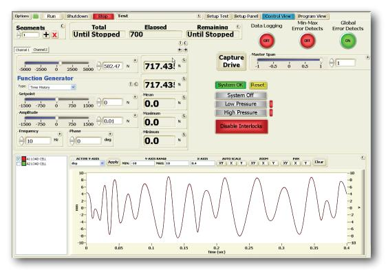
The centerpiece of the SWCS is the Multi Axis Function Generator. This is where users will spend most of their time. The function generator is a powerful test programming environment, complete with sophisticated Real Time Active Control (RTAC), that optimizes the commands, so that the system accurately responds with the signal you intend. The Multi-Axis Function Generator can reproduce the following signals:
